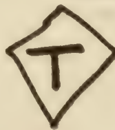
Abrupt end of Road
