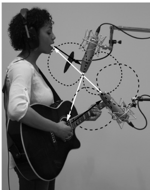
Figure 9.4 The angles and distances from the mics to their respective sound sources are changed to keep them more on axis with their desired sources while aiming their null points at the sources of spill.
