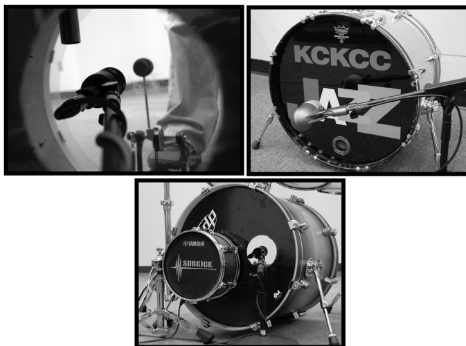
Figure 10.1 Top Left: Looking through the hole into a kick drum with a mic typically placed for single mic recording, several inches from the beater-side head. Top Right: A mic about 15 cm (6 in) outside the center of a jazz kick drum. Avoid miking at or close to the outside of a hole as small as the one in this drum – a very strong air current is forced through a hole this small. Bottom: A combination of a sub-kick mic, and a conventional mic inside the drum.
