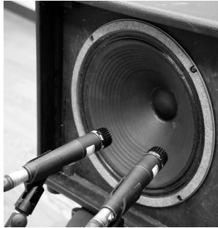
Figure 11.1 A guitar cabinet loudspeaker miked on-axis for the brightest sound, and off-axis for a warmer sound.
