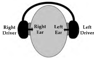
Figure 2.3 A binaural headphone or earbud system lacks the inter-aural crosstalk necessary to make it a true stereo system.
