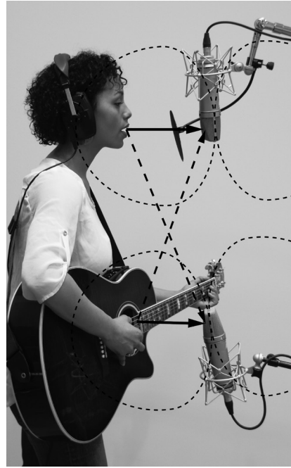
Figure 9.3 Using bidirectional mics on-axis to their desired sound source reduces spill, but the nulls are not quite aligned with the respective sources of spill, so rejection is not maximized.
