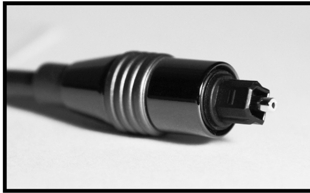
Figure 1.25 A TOSLINK optical fiber connector as used for optical SPDIF connections.
