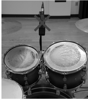
Figure 10.5 Not recommended! This cardioid mic is off-axis to both drums! The sound will lack attack and punch, and the drums cannot be individually panned or processed.
