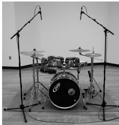
Figure 10.6 A spaced array with a mic positioned over each bank of cymbals, at the first and third “quarter” divisions of the width of the set.
