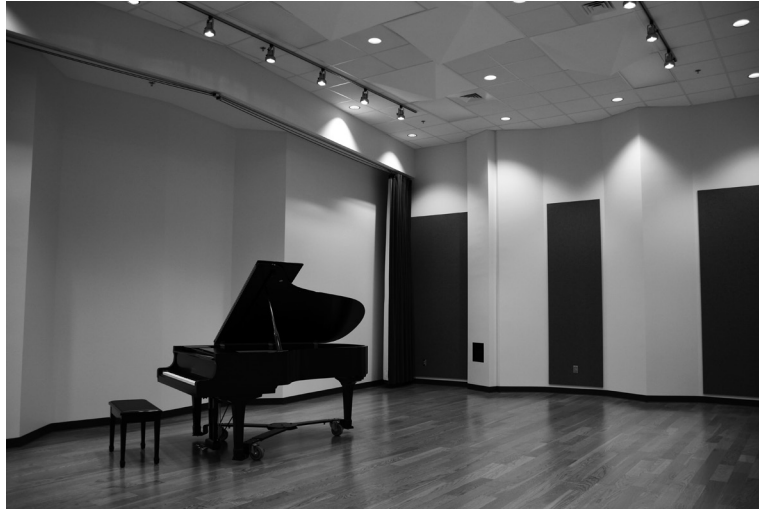
Figure 8.1 A live room with hard, reflective surfaces that reflect the sound back into the room towards the mics and performers. (Kansas City Kansas Community College, Kansas City, KS).
