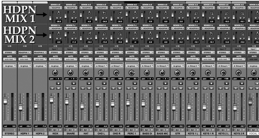
Figure 16.1 Stereo sends used for multiple headphone monitor mixes in a DAW. Two sends (SENDS e and f, the top two small faders of each channel) are assigned across all tracks, with different mixes (amplitude and panning) dialed in for each. On the left of the mix window are the master faders for the main stereo mix, and the two headphone mixes.
