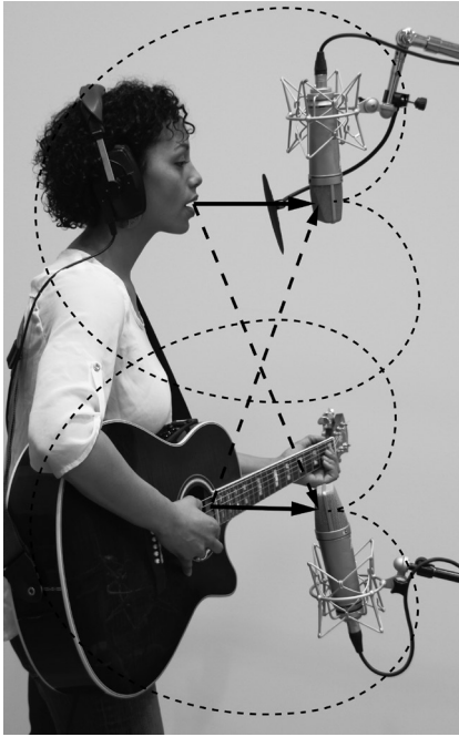
Figure 9.2 A singer/guitarist miked with cardioid mics. Each mic picks up significant off-axis (colored) spill.
