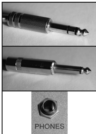
Figure 1.21 Top: A quarter-inch TRS male plug. Middle: A quarter-inch TS male plug. Bottom: A quarter-inch female socket/jack (it could be TS or TRS – there’s no way to tell visually, but “Phones” here indicates that it is TRS).
