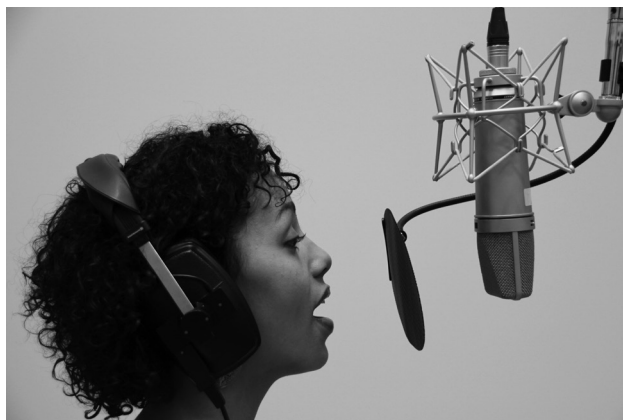
Figure 3.17 A correctly positioned pop filter, with a few inches of distance between the singer and the filter, and the filter and the microphone.
