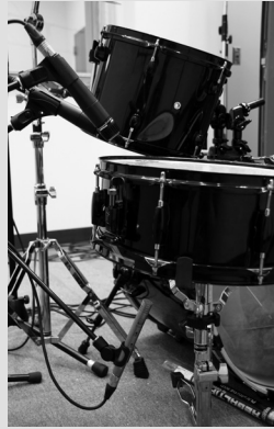
Figure 10.2 A double miked snare drum (dynamic mic on the top, small diaphragm condenser on the bottom) showing the different top mic angles described in the main text. (You would not normally use two identical mics at different angles simultaneously.) The mic stands are boomed in from behind the snare drum, in-between the tom tom and hi-hat. (The hi-hat is not shown in this picture because it would obscure the mics in the picture.)
