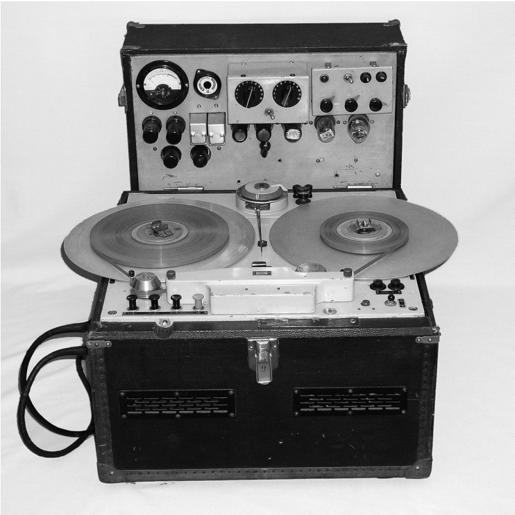
FIGURE 5.2 AEG Magnetophon type K4 sp, advanced AC biased tape recorder with 6.5 mm ferric coated I.G. Farben tape. One of two shipped back by Jack Mullin at the end of World War II.
